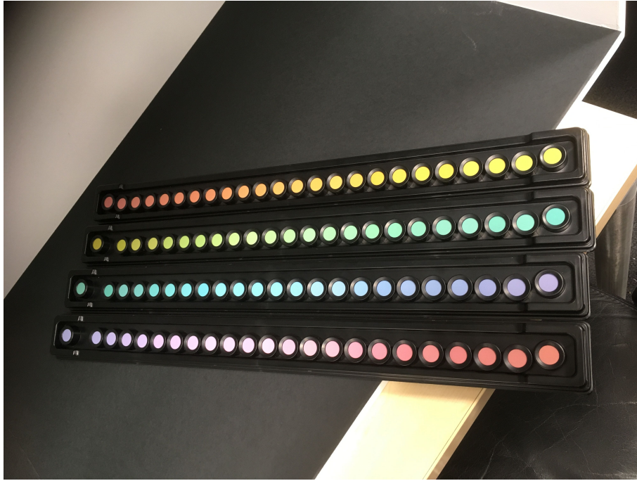
Figure 3.12: The FM100-hue test with tray 1, tray 2, tray 3 and tray 4 from top to bottom.
